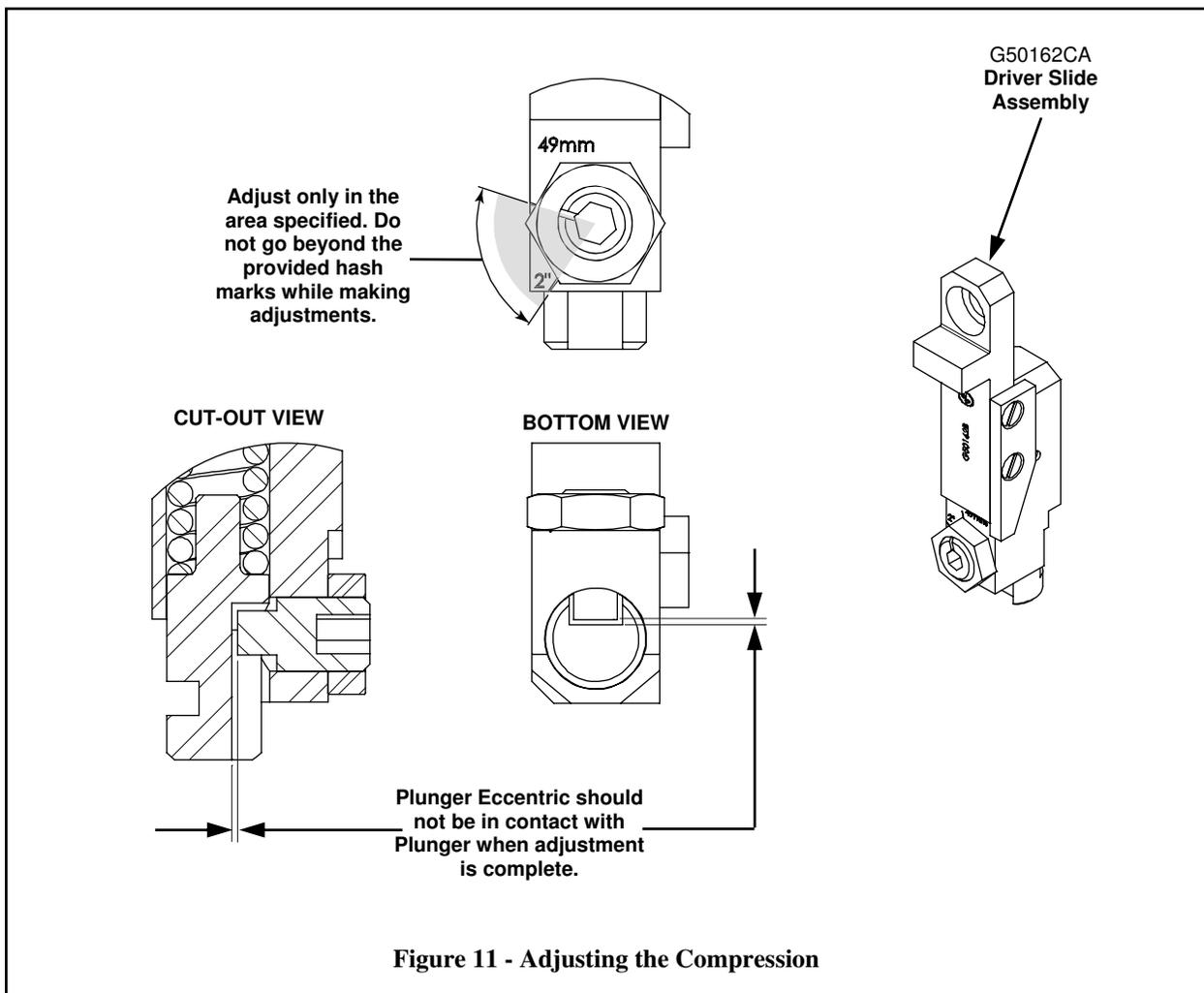
Figure 11 - Adjusting the Compression
